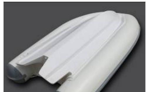
ST 280 / ST 260: nuova carena alte prestazioni con flaps integrati / new high perform. hull with integrated flaps
